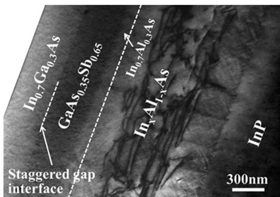
FIG. 2. Cross-sectional TEM micrograph of the entire TFET layer structure with 150 nm intrinsic In<sub>0.7</sub>Ga<sub>0.3</sub>As channel and 200 nm n<sup>+</sup> In<sub>0.7</sub>Ga<sub>0.3</sub>As drain layer. No threading dislocations were detected in the In<sub>0.7</sub>Ga<sub>0.3</sub>As and GaAs<sub>0.35</sub>Sb<sub>0.65</sub> layers, indicating high crystalline quality of the active region.
