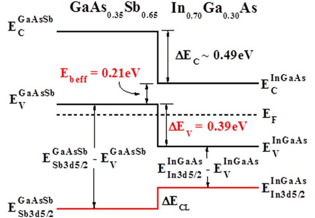
FIG. 5. Schematic of the energy-band diagram of  $\text{GaAs}_{0.35}\text{Sb}_{0.65}/\text{In}_{0.7}\text{Ga}_{0.3}\text{As}$  heterointerface in an n-channel TFET structure. A type-II staggered band alignment with an effective tunneling barrier height of  $0.21\text{ eV}$  was measured at the heterointerface.
