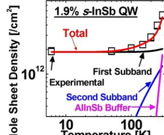
Fig.5: Experimental and modeled hole sheet density as a function of temperature for InSb QW heterostructure. Showing contributions from first and second lh subband and AlInSb buffer layer conduction at room temperature.
