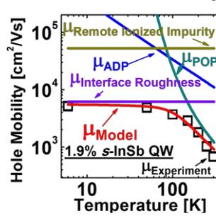
Fig.6: Experimental and modeled hole hall mobility as a function of temperature for InSb QW heterostructure.
