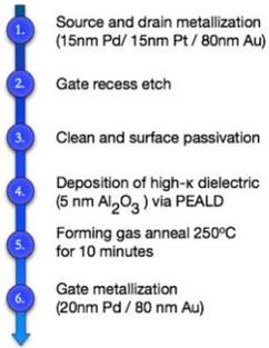
Fig.8: Fabrication process flow for InSb QW-MOSFET.
