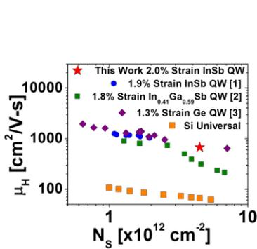
Fig.1: Hall hole mobility versus hole sheet density at  $T=300\text{K}$  for Si, Ge, QW, InGaSb, and InSb QWs heterostructures.
