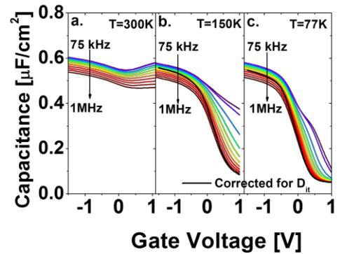
Fig.10: Measured split CV characteristics for (a)  $300\text{K}$ . Measured split CV and corrected for  $D_{it}$  split CV characteristics for (b)  $150\text{K}$ , and (c)  $77\text{K}$ .
