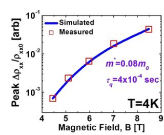
Fig.4: Modeled and experimental peak  $\Delta\rho_{xx}/\rho_{xx0}$  as a function of magnetic field used to extract the effective mass and quantum lifetime for the InSb QW heterostructure.
