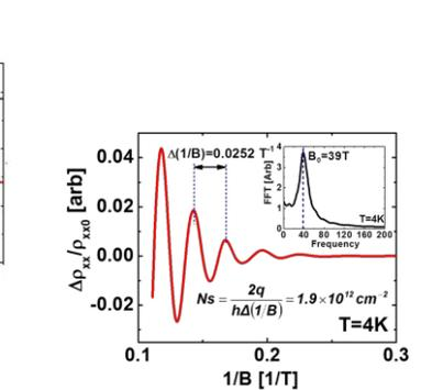
Fig.3: Shubnikov-de Haas oscillations in sheet resistance as a function of  $1/B$  at  $T=4\text{K}$ , inset shows FFT of the oscillations showing single frequency peak at  $39\text{T}$ , indicating that only one hh subband is occupied at this sheet charge.
