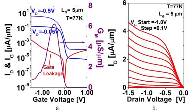
Fig.11: (a)  $I_D$ - $V_G$  characteristics for  $L_G = 5\ \mu\text{m}$  InSb QW-MOSFET at  $T=77\text{K}$ . The device exhibits  $I_{ON}$  of  $2.0\ \mu\text{A}/\mu\text{m}$ , a peak  $G_{mSat}$  of  $6.8\ \mu\text{S}/\mu\text{m}$  and a SS of  $58\ \text{mV}/\text{dec}$ . (b)  $I_D$ - $V_D$  characteristics for  $L_G = 5\ \mu\text{m}$  InSb QW-MOSFET at  $T=77\text{K}$
