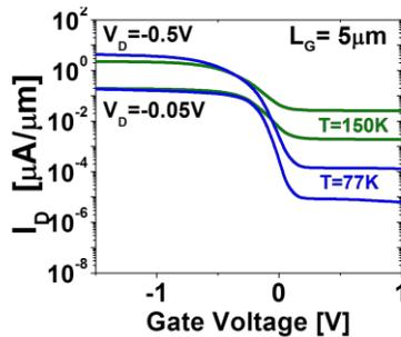
Fig.12:  $I_D$ - $V_G$  characteristics for  $L_G = 5\ \mu\text{m}$  InSb QW-MOSFET as a function of temperature for  $V_D = -50\text{mV}$  and  $V_D = -0.5\text{V}$ .
