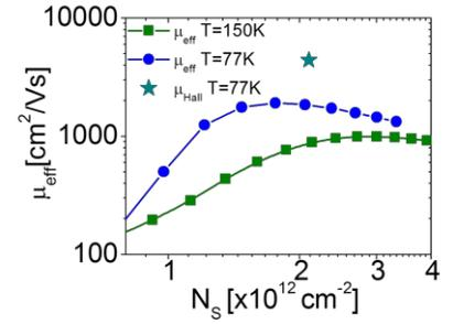
Fig.13: Extracted effective mobility as a function of carrier density at  $T=77\text{K}$  and  $T=150\text{K}$  compared with Hall mobility at  $77\text{K}$ .
