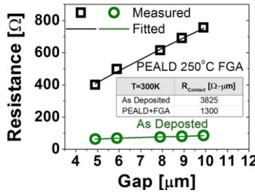
Fig.9: Circular TLM measurements following contact deposition, after PEALD  $\text{Al}_2\text{O}_3$  deposition and FGA.
