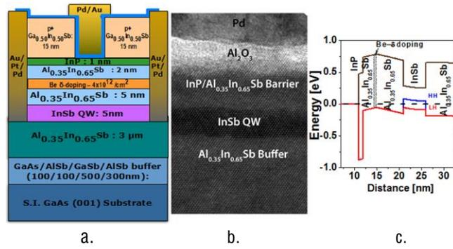
Fig.2: (a) Schematic of InSb QW-MOSFET on S.I. GaAs substrate with 5nm PEALD  $\text{Al}_2\text{O}_3$  (b) Cross-sectional TEM micrograph on InSb-MOSFET gated region (c) Energy band diagram of the quantum well heterostructure. Simulated using 6-band k.p Schrodinger-Poisson self-consistent solver.
