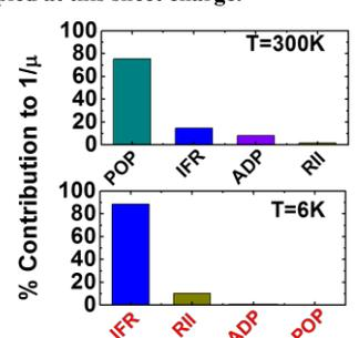
Fig.7: Pareto plot showing % contribution and dominant scattering mechanisms at  $T=300\text{K}$  and  $T=6\text{K}$ .
