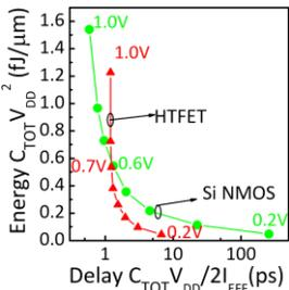
Fig. 7 Switching energy-delay for FOI inverter using effective current ( $I_{EFF}$ ) evaluation. Cross-over happens at  $V_{DD}=0.6\text{V}$  for NMOS. HTFET shows lower power advantage below  $0.6\text{V}$ .
