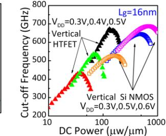
Fig. 8  $F_T$ -DC power of vertical HTFET and Si NMOS of  $L_g=16\text{nm}$ . HTFET shows superior high frequency performance at low DC power.
