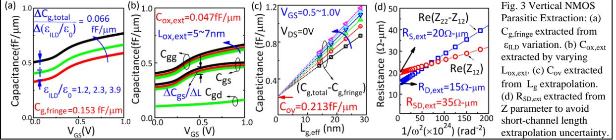
Fig. 3 Vertical NMOS Parasitic Extraction: (a)  $C_{g,fringe}$  extracted from  $\epsilon_{ILD}$  variation. (b)  $C_{ox,ext}$  extracted by varying  $L_{ox,ext}$ . (c)  $C_{ov}$  extracted from  $L_g$  extrapolation. (d)  $R_{SD,ext}$  extracted from Z parameter to avoid short-channel length extrapolation uncertainty.
