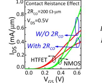
Fig. 9 Contact resistance ( $R_{CO}$ ) effect on vertical HTFET and Si NMOS. HTFET shows lower current degradation (26%) with large  $R_{CO}$  than NMOS (40%) due to high tunneling resistance.
