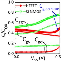
Fig. 5 Normalized capacitance comparison of vertical NMOS and HTFET at  $V_{DD}=0.5\text{V}$ . Lower  $C_g$  in HTFET comes from lower drain doping.
