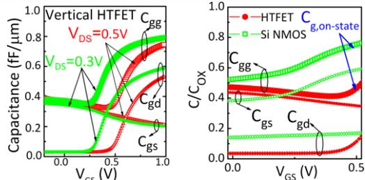
Fig. 4 C-V plots of HTFETs at  $V_{DS} = 0.3\text{V}$ ,  $0.5\text{V}$ . At low  $V_{GS}$ ,  $C_{gg}$  is dominant by  $C_{gs}$ . As  $V_{GS}$  increases,  $C_{gd}$  dominates as on-state enhanced  $C_{miller}$ .
