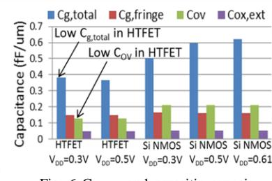
Fig. 6  $C_{g,total}$  and parasitic capacitance comparison of vertical HTFET and Si NMOS. HTFET presents lower  $C_{g,total}$  and reduced  $C_{ov}$  compared to Si NMOS.
