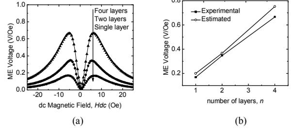
Figure 3. (a) ME voltage of the sensor system as a function of dc bias magnetic field for Metglas/PVDF laminates with different number of PVDF layers. The data were measured at 200 Hz and ac magnetic field  $H_{ac}=0.08 \text{ Oe}$ . The feedback capacitance in charge amplifier is 10 pF. (b) Comparison of experimentally measured ME voltage with that deduced (estimated) from (5).
