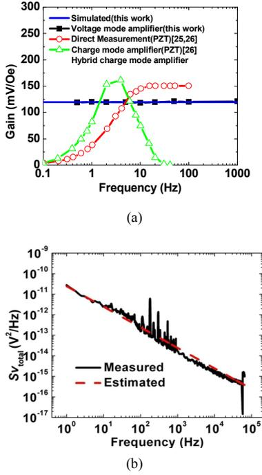
Figure 6. Output response of voltage mode sensing system (a) Frequency response and its comparison with other detection techniques, (b) Calculated and measured total input noise power spectral density.
