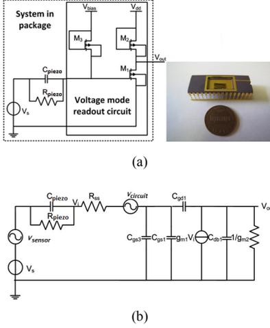
Figure 2. (a) Schematic and photography for SIP ME laminates sensor and voltage mode readout circuit, (b) Small signal circuit for voltage mode ME system with noise sources.
