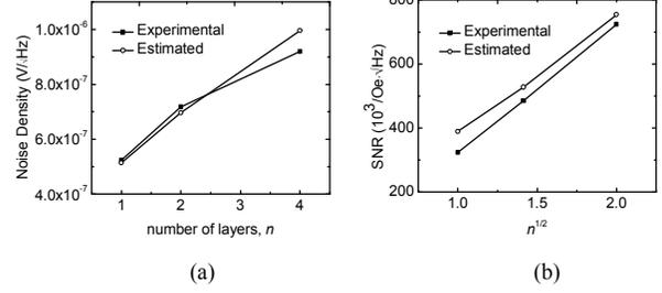
Figure 5. (a) Output referred noise density at 200 Hz as a function of the number of PVDF layers (dots) and its comparison with that deduced (open circles) from (8), (b) SNR at 200 Hz as a function of the square root of the number of PVDF layers (dots) and the comparison with that deduced from (9) (open circles). Lines are drawn to guide eyes.
