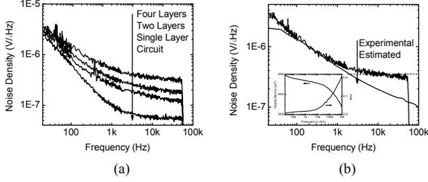
Figure 4. (a) Noise spectral density for Metglas/PVDF laminates with varying number of PVDF layers, (b) Comparison of the experimentally measured noise spectral density for laminates with four layers PVDF with that deduced from (8). (The inset shows the capacitance and  $\tan\delta$  of the PVDF as a function of frequency which are used in the calculation).
