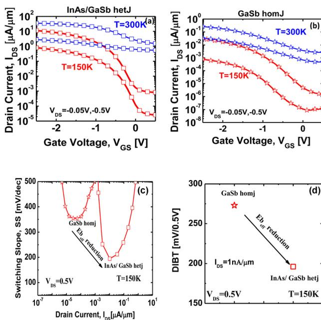
FIG. 6. (a) and (b)  $I_{DS}-V_{GS}$  characteristics of hetJ and homJ pTFETs at  $T = 300\text{ K}$  and  $150\text{ K}$ . (c) SS as a function of drain current at  $T = 150\text{ K}$  showing lower SS in hetJ compared to homJ pTFET. (d) hetJ pTFET exhibits lower DIBT compared to homJ pTFET at  $I_{DS} = 1\text{ nA}/\mu\text{m}$ ,  $T = 150\text{ K}$ .
