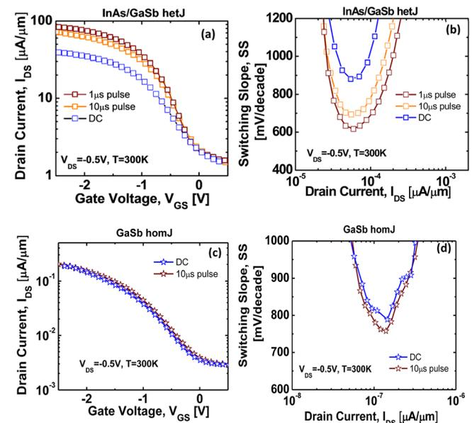
FIG. 7. (a)  $I_{DS}-V_{GS}$  characteristics of hetJ for varying gate voltage pulse widths. (b) SS of hetJ pTFET as a function of drain current for varying gate voltage pulse widths. (c)  $I_{DS}-V_{GS}$  characteristics of homJ pTFET show negligible change in  $I_{ON}$  with  $10\ \mu\text{s}$  gate voltage pulsing compared to DC bias conditions. (d) SS of homJ pTFET shows negligible change in  $I_{ON}$  with  $10\ \mu\text{s}$  gate voltage pulsing compared to DC bias conditions.
