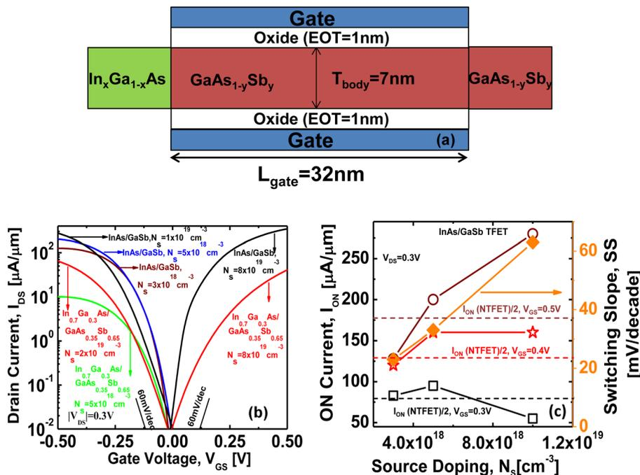
FIG. 2. (a) Schematic of ultra-thin body pTFET simulated. (b) Transfer characteristics of InAs/GaSb and  $\text{In}_{0.7}\text{Ga}_{0.3}\text{As}/\text{GaAs}_{0.35}\text{Sb}_{0.65}$  pTFET as a function of the source doping. (c)  $I_{\text{ON}}$  as a function of  $N_{\text{S}}$  in InAs/GaSb pTFET.
