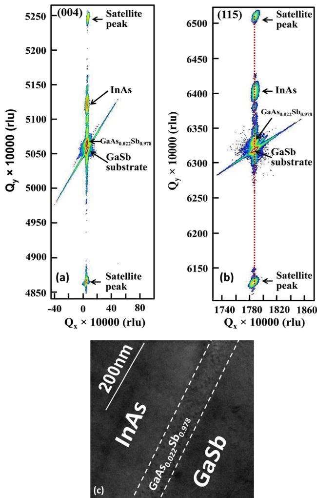
FIG. 8. (a) and (b) Symmetric and asymmetric RSM of InAs/GaSb structure showing the presence of GaAs<sub>0.022</sub>Sb<sub>0.978</sub> at the hetero-junction. (c) Cross-section TEM of the InAs/GaSb structure confirming the presence of an amorphous layer of GaAs<sub>0.022</sub>Sb<sub>0.978</sub> at the hetero-junction.
