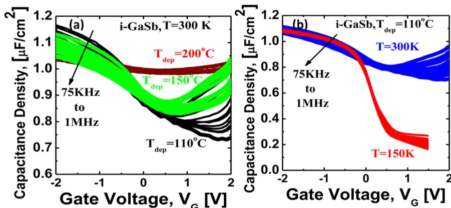
FIG. 4. (a) C–V characteristics of Al<sub>2</sub>O<sub>3</sub>/HfO<sub>2</sub> deposited on p-type GaSb in the frequency range of 75 KHz to 1 MHz measured at 300 K as a function of deposition temperature. (b) C–V characteristics of Al<sub>2</sub>O<sub>3</sub>/HfO<sub>2</sub> deposited 110 °C and measured at  $T = 300$  K and  $T = 150$  K.
