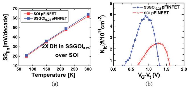
Fig. 4. (a) Subthreshold slope as a function of temperature at  $V_{ds} = -50$  mV shows higher interface state density in SSGOI<sub>0.25</sub> than in SOI. (b) Measured interface state profile via charge pumping measurements.
