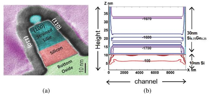
Fig. 1. (a) Cross-sectional TEM micrograph of the SiGe/Si stacked fin under the gate with 30 nm of  $\text{Si}_{0.75}\text{Ge}_{0.25}$  and 10 nm of Si. (b) FEM simulation of 10- $\mu\text{m}$ -long SSGOI<sub>0.25</sub> pFINFET shows a compressive average sidewall stress of  $\sim 1.6$  GPa.
