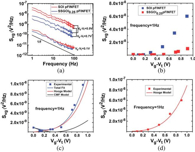
Fig. 2. (a) Gate referred flicker noise for both SSGOI<sub>0.25</sub> and SOI shows slope of close to 1. (b) Comparison of  $S_{vg}$  as a function of gate overdrive voltage shows that SSGOI<sub>0.25</sub> FINFETs have lower noise levels compared to SOI FINFETs. (c) CMF is dominant in the low-gate-bias range and the Hooge model is dominant in the high-gate-bias range in SSGOI<sub>0.25</sub> pFINFETs. (d) Hooge model covers the entire gate-bias range in SOI pFINFETs.
