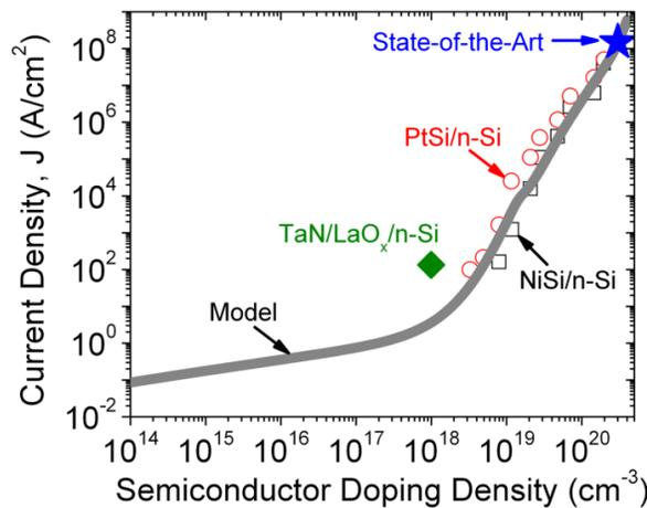
**Fig. 5** Benchmarking of TaN/LaO<sub>x</sub>/*n*-Si contact architecture [2] versus NiSi/*n*-Si reference.
