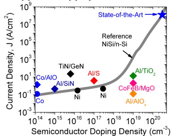
**Fig. 6** Benchmarking of various contact architectures on *n*-Germanium [1, 7-10] versus NiSi/*n*-Si reference.
