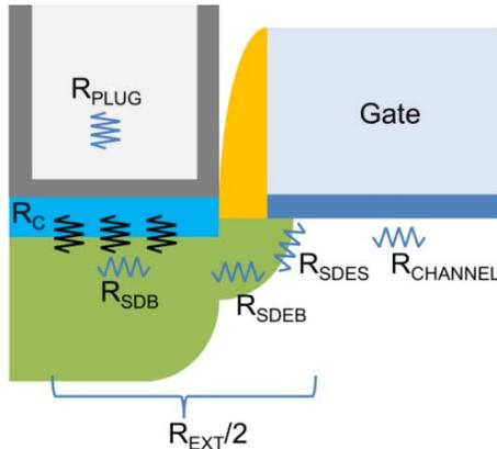
**Fig. 1** Schematic showing different resistance components in a MOSFET. Interface contact resistance ( $R_C$ ) is one of the biggest challenges facing CMOS performance and power scaling due to contact length scaling in accordance with Moore's law (See Fig. 2).
