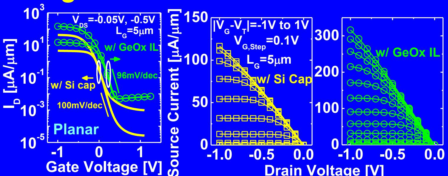
**Ge QW/Si Cap or GeO<sub>x</sub> IL/5Å Al<sub>2</sub>O<sub>3</sub>/22Å HfO<sub>2</sub>**
