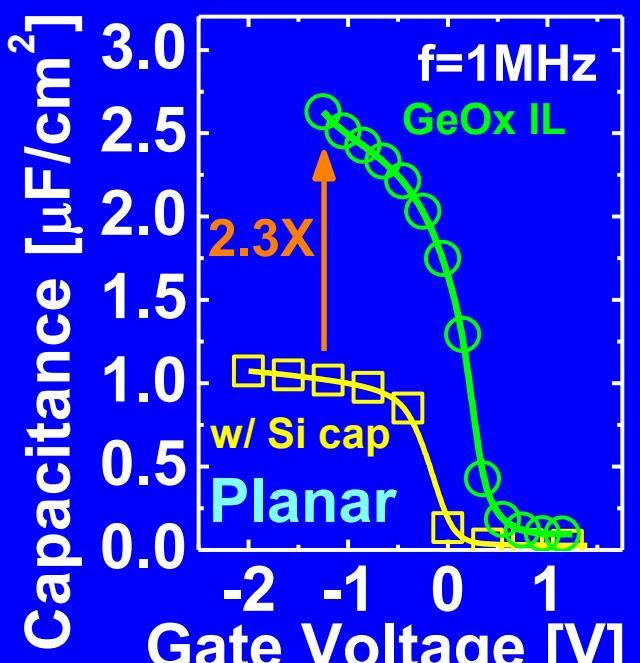
**Ge QW/6A GeOx IL/5A  $\text{Al}_2\text{O}_3/22A \text{HfO}_2$**
