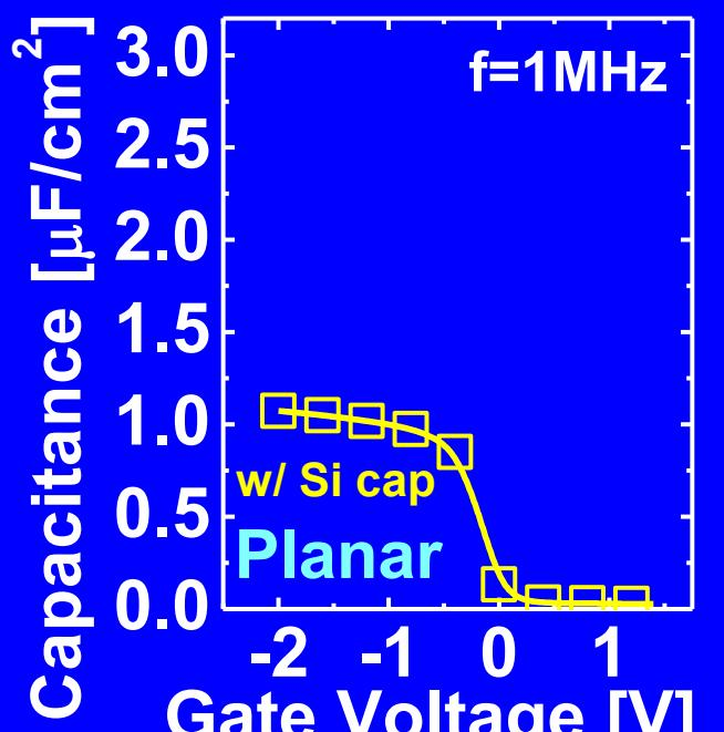
Ge QW/10A Si cap/5A Al<sub>2</sub>O<sub>3</sub>/22A HfO<sub>2</sub>
