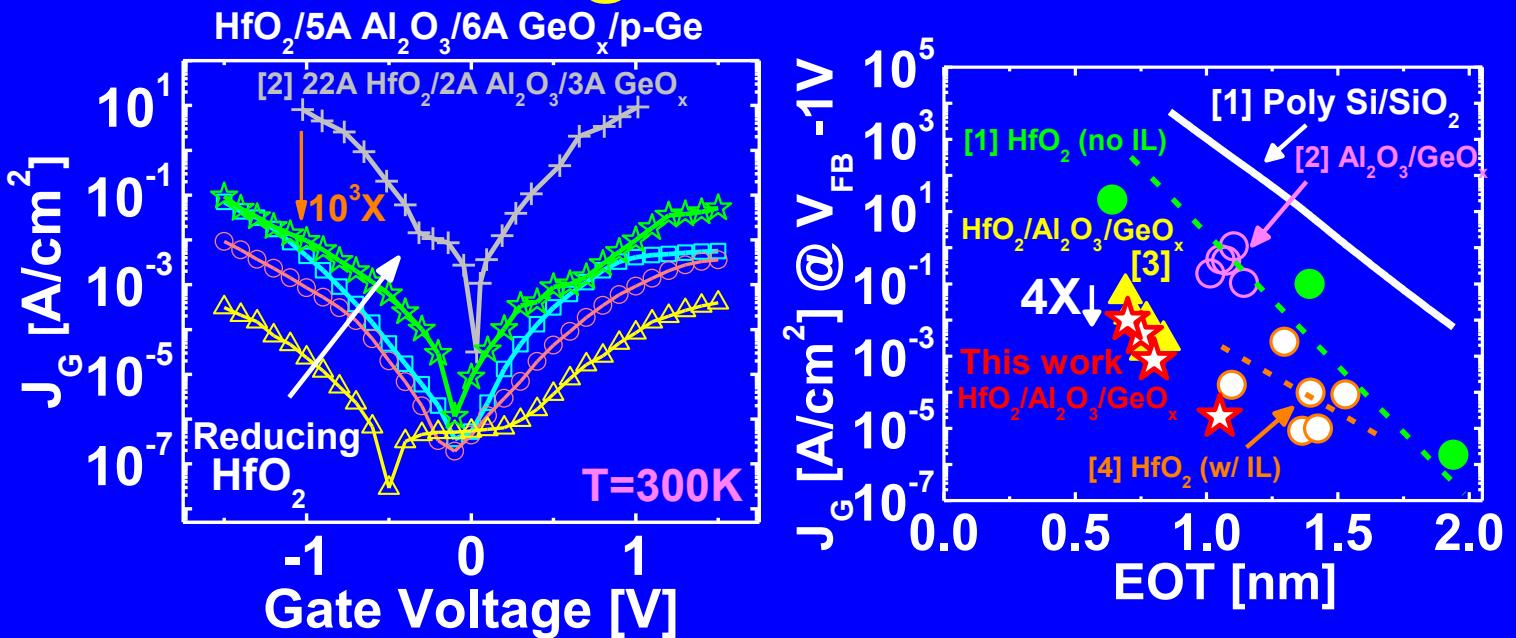
➤ Low gate leakage of  $10^{-2} \text{ A}/\text{cm}^2$  ( $V_G = V_{FB} - 1\text{V}$ ) obtained at 0.72nm EOT with Tri-layer gate stack
