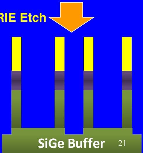
➤ FinFET fabrication using Sidewall Image Transfer (SIT)
