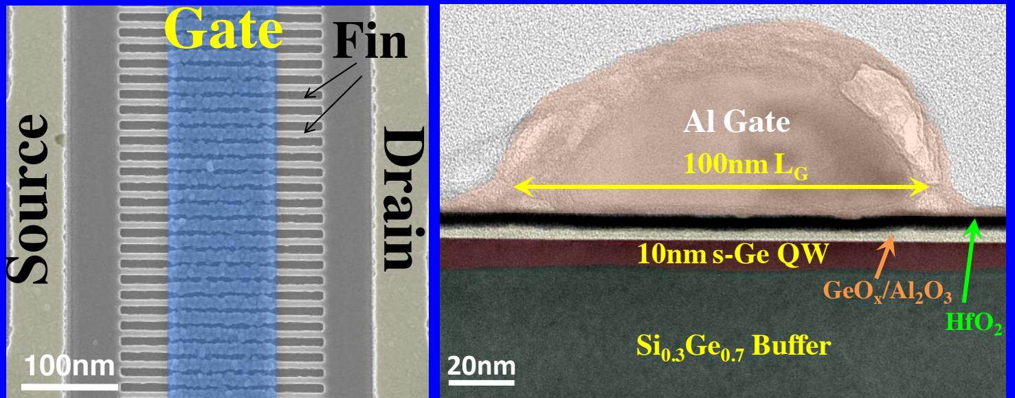
➤ Short channel FinFET with gate length of 100nm and Tri-layer high- $\kappa$  fabricated using SIT
