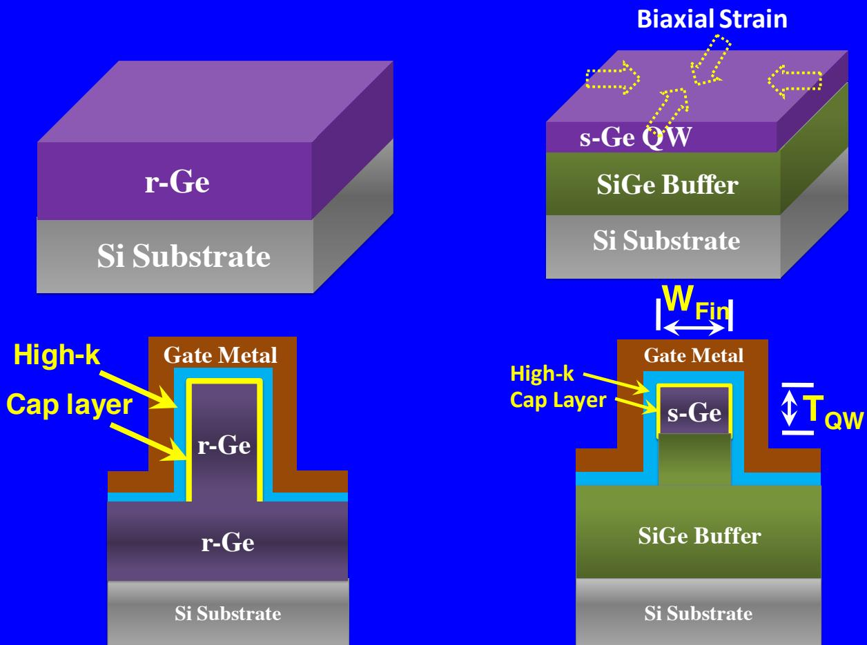
➤ Both  $W_{fin}$  and  $T_{QW}$  determine strain in Ge QW <sup>6</sup>
