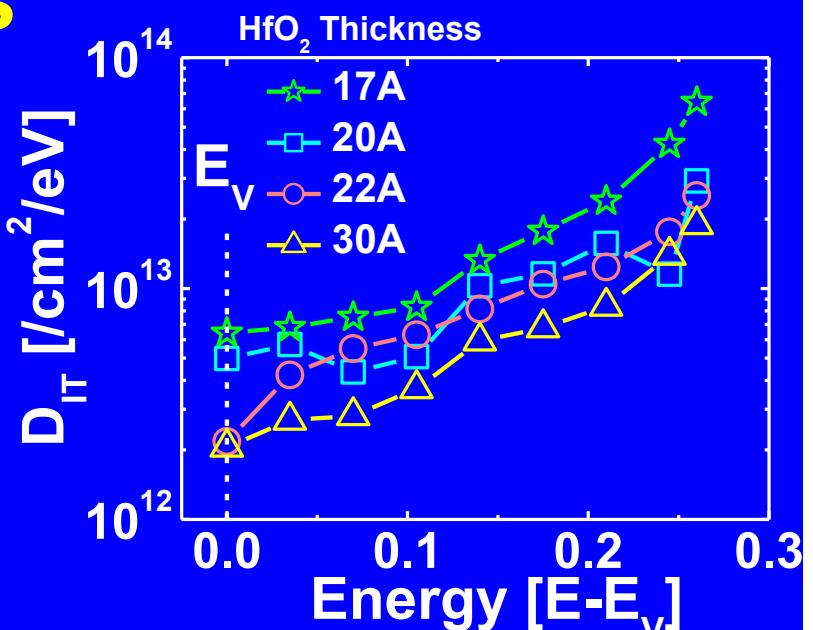
**HfO<sub>2</sub>/5A Al<sub>2</sub>O<sub>3</sub>/6A GeO<sub>x</sub>/p-Ge**
