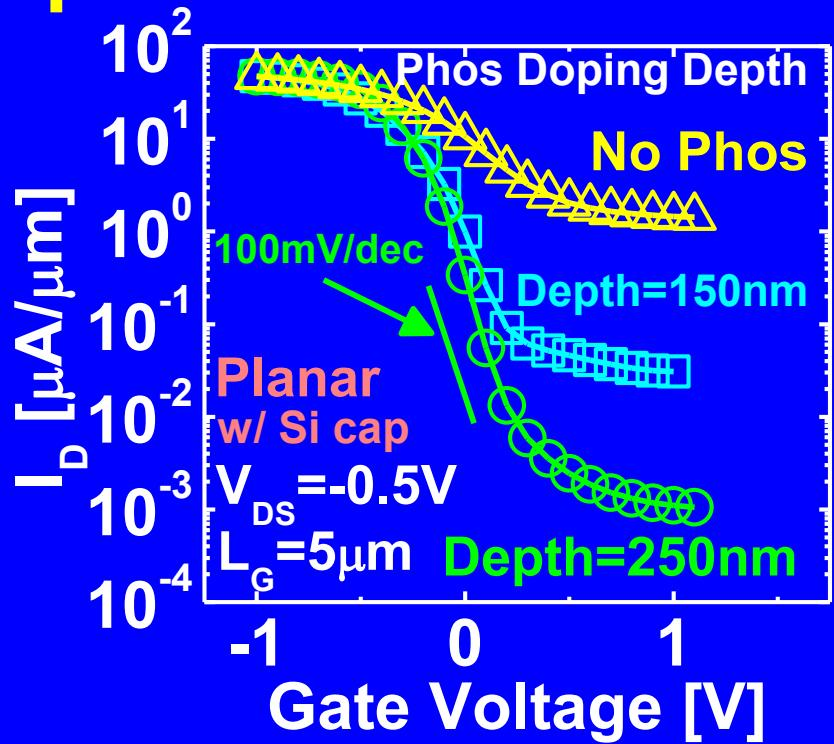
➤  $10^3 \times I_{OFF}$  reduction with deeper Phos doping in SiGe buffer with no degradation in  $I_{ON}$
