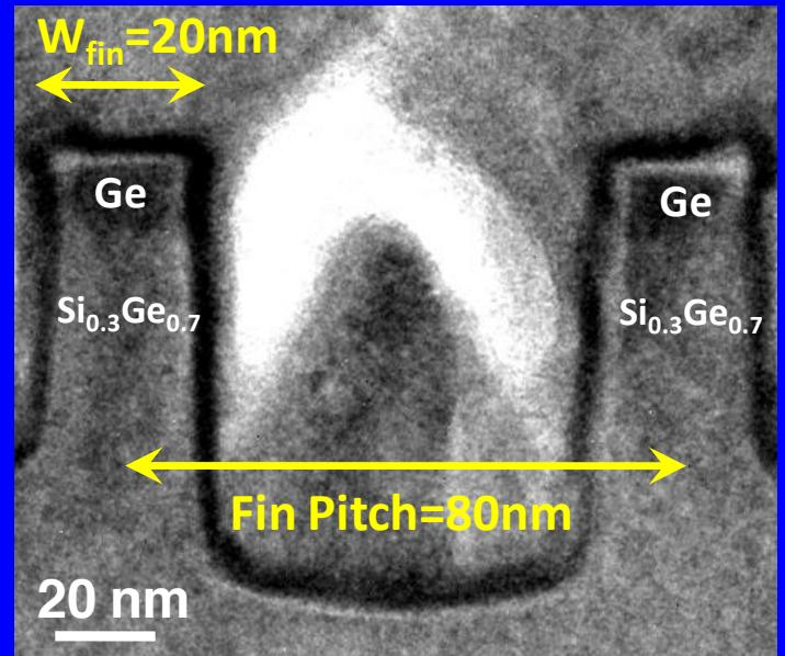
➤  $W_{fin}=20\text{nm}$ ; Fin pitch = 80nm; Tri-layer high- $\kappa$  realized on s-Ge QW with SIT process
