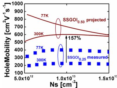
Fig 7. Measured and predicted hole mobilities in SiGe FINETs
