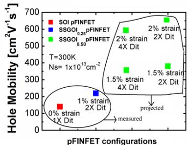
Fig 10. Measured and projected hole mobilities in SiGe FINETs
