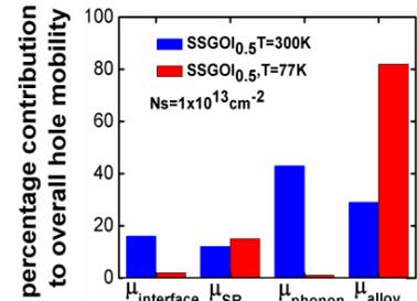
Fig 8. Alloy scattering is the single dominant mechanism at 77K in SSGOI<sub>0.5</sub> FINET
