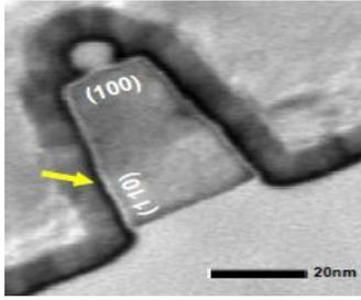
Fig 1. Cross section of SiGe/Si stack fin under gate with Si<sub>0.75</sub>Ge<sub>0.25</sub>(30nm)/Si(10nm)
