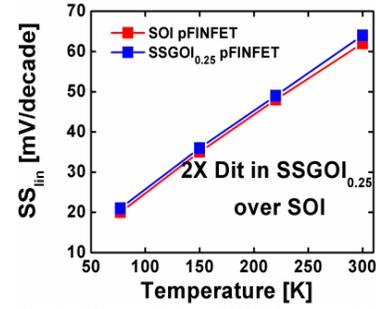
Fig 3. SS<sub>lin</sub> vs T for SSGOI<sub>0.25</sub> and SOI pFETs
