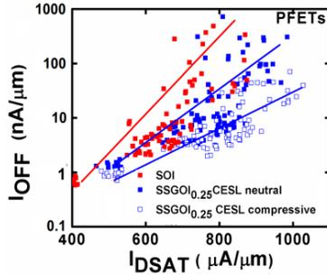
Fig 2. Ioff vs Idsat shows better performance of SSGOI<sub>0.25</sub> over SOI pFETs
