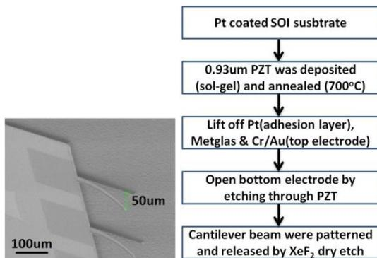
Fig. 2 SEM and process flow for ME cantilevers.
