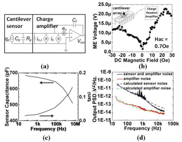
Fig. 4 (a) Equivalent circuit with noise source (b) ME cantilever output voltage versus DC magnetic field (input ac magnetic field equals 0.7 Oe) (c) Sensor capacitance and dielectric loss vs. frequency (d) noise power spectrum density (PSD) of amplifier and sensor
