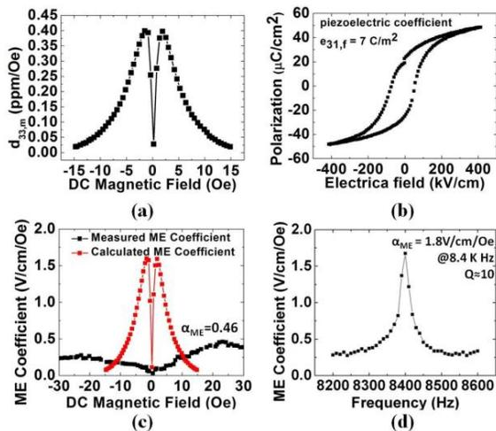
Fig. 3 ME cantilever characterization: (a) Magnetostriction of Metglas (b) PE loop & piezo coefficient of PZT (c) Measurement vs. calculated ME coefficient (d) ME coefficient at resonance (8.4 K Hz)
