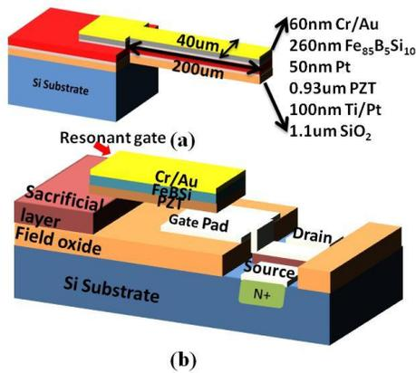
Fig. 1 Schematic for Magnetolectric (ME) (a) cantilever and (b) resonant gate transistor (RGT).
