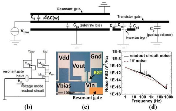
Fig. 5 (a) Equivalent circuit of ME RGT (b) Voltage mode readout circuit diagram (c) ME RGT readout circuit layout (d) Noise PSD for the readout circuit
