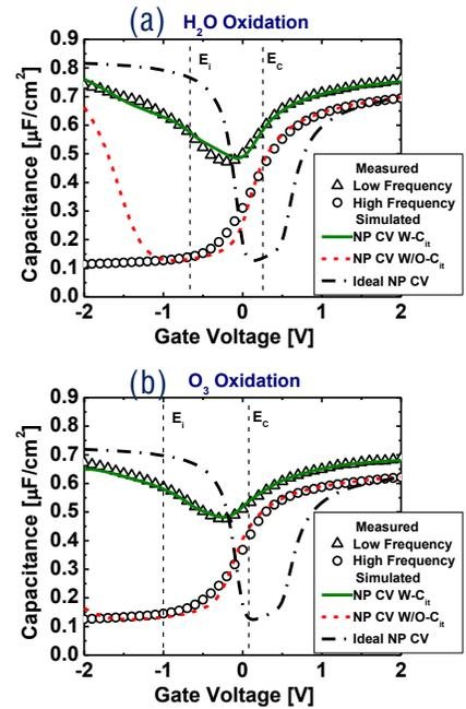
Fig.4: Measured true Low and High frequency fitted with calculated C-V with  $D_{it}$  for ntype In<sub>0.53</sub>Ga<sub>0.47</sub>As Moscap with (a) H<sub>2</sub>O and (b) O<sub>3</sub> based ALD Al<sub>2</sub>O<sub>3</sub>.
