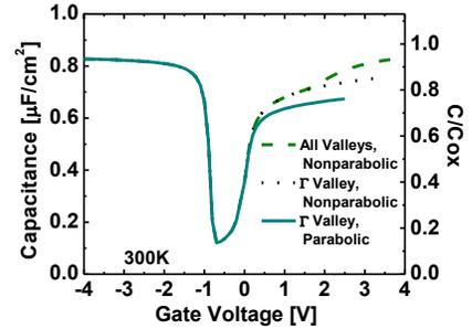
Fig.3: Simulated capacitance showing the effect of non parabolic approximation and satellite valley for In<sub>0.53</sub>Ga<sub>0.47</sub>As with 8nm Al<sub>2</sub>O<sub>3</sub> high-κ (ε<sub>r</sub>~8) as a function of gate bias.
