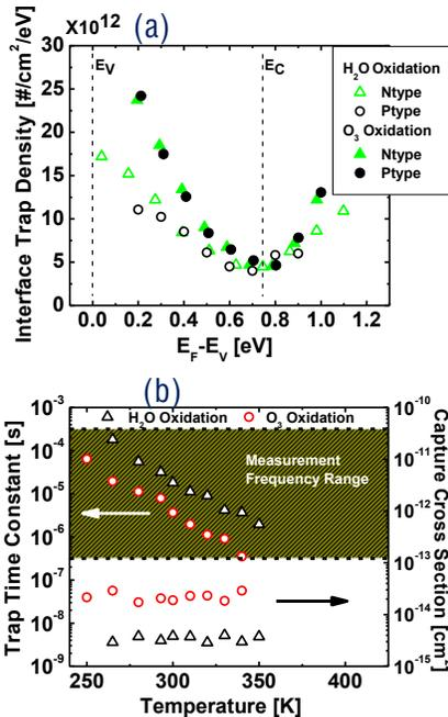
Fig.5: Extracted (a) interface trap density and (b) interface trap time constant and capture cross section at  $E_F \sim E_g/2$  for the water and ozone based ALD Al<sub>2</sub>O<sub>3</sub>.
