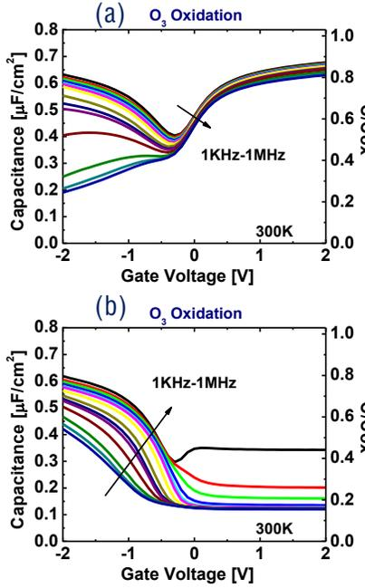
Fig.2: C-V characteristics as a function of frequency of (a) ntype and (b) ptype In<sub>0.53</sub>Ga<sub>0.47</sub>As Moscap with O<sub>3</sub> based ALD Al<sub>2</sub>O<sub>3</sub>.
