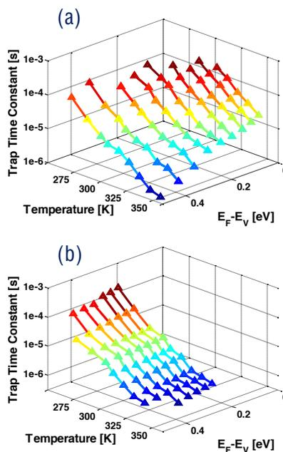
Fig.6: Trap time constant as a function of energy and temperature for (a) H<sub>2</sub>O and (b) O<sub>3</sub> based ALD Al<sub>2</sub>O<sub>3</sub>.
