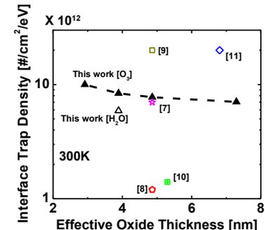
Fig.7: Midgap  $D_{it}$  evaluated by conductance method at room temperature compared with other work reported in literature.
