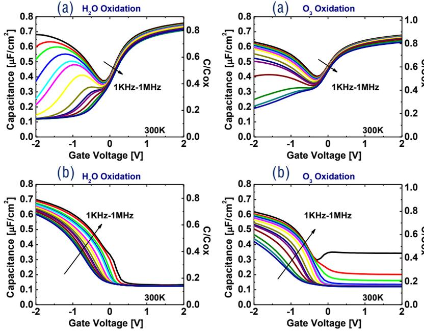
Fig.1: C-V characteristics as a function of frequency of (a) ntype and (b) ptype In<sub>0.53</sub>Ga<sub>0.47</sub>As Moscap with H<sub>2</sub>O based ALD Al<sub>2</sub>O<sub>3</sub>.
