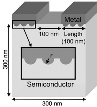
**Figure 1.** Three-dimensional depiction of the structure used for the simulations, showing the circular features at the metal-semiconductor interface. In three dimensions, the circular features become rods running the width of the contact.
