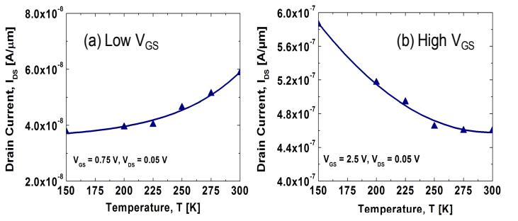
**Fig 8.**  $In_{0.53}Ga_{0.47}As$  TFET on current (a) increases at low  $V_{GS}$  due to reducing tunnel gap (limited by tunnel barrier resistance) and (b) decreases with temperature at high  $V_{GS}$  (limited by phonon scattering limited channel resistance).
