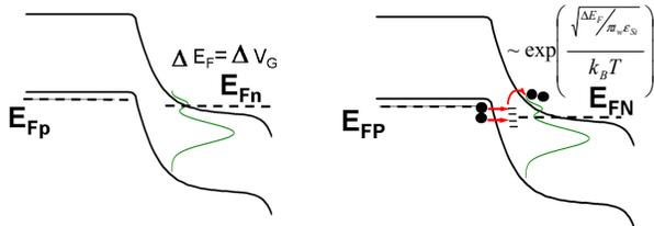
**Fig 6.** Energy band diagrams illustrating the impact of  $D_{it}$  on TFET sub-threshold slope; (a)  $D_{it}$  only effect is negligible and (b)  $D_{it}$  and TAT degrades sub-threshold slope since it involves tunneling into the interface traps and subsequent thermal emission from the traps giving rise to temperature dependence.
