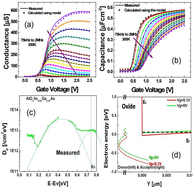
**Fig 5.** Measured (a) conductance, (b) capacitance, (c) interface state profile ( $D_{it}$ ) for  $\text{In}_{0.53}\text{Ga}_{0.47}\text{As}$  MOSFET and (d) simulated movement of Fermi level across  $D_{it}$  profile for  $\text{In}_{0.53}\text{Ga}_{0.47}\text{As}$  TFET.
