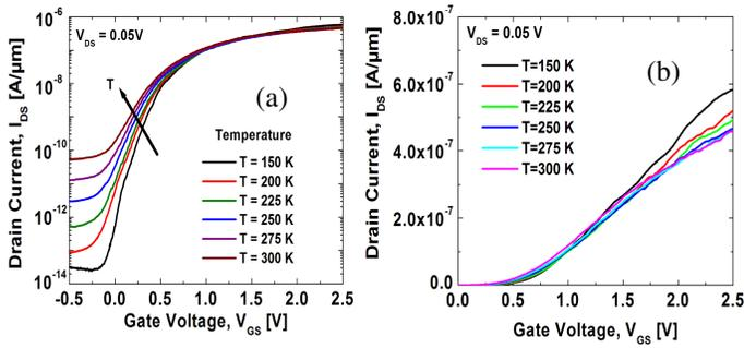
**Fig 7.**  $\text{In}_{0.53}\text{Ga}_{0.47}\text{As}$  TFET transfer characteristics illustrating the temperature dependence of the leakage floor and the on-current. The leakage floor increases exponentially with increasing temperature consistent with SRH generation recombination mechanism.
