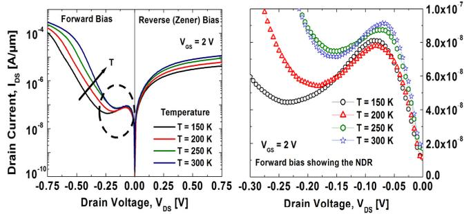
**Fig 9.** Gated negative differential resistance (NDR) characteristics as a function of temperature during forward bias between drain and source of  $\text{In}_{0.53}\text{Ga}_{0.47}\text{As}$  TFET. A PVCR of 2 is observed at 150K.
