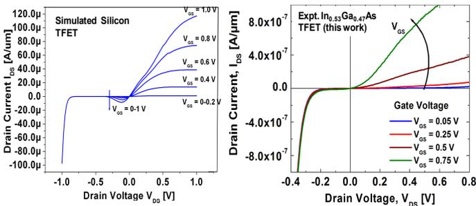
**Fig 11.** Asymmetric output characteristics in Si TFETs (simulated) and experimentally observed in  $\text{In}_{0.53}\text{Ga}_{0.47}\text{As}$  TFETs due to the inherent diode between source and drain, highlighting the difficulty in pass transistor implementation.
