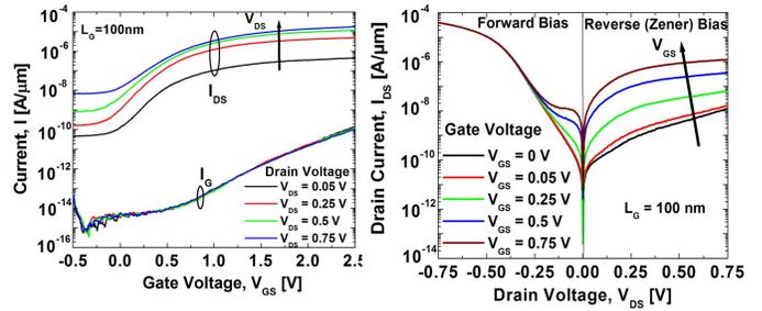
**Fig 2.** Measured (a)  $I_D-V_{GS}$ ,  $I_G-V_{GS}$  and (b)  $I_D-V_{DS}$  characteristics for a 100nm channel length vertical  $\text{In}_{0.53}\text{Ga}_{0.47}\text{As}$  TFET.
