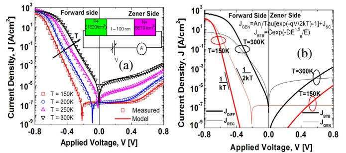
**Fig 3.** (a) Measured and modeled  $J-V$  characteristic and (b) various modeled components for  $\text{In}_{0.53}\text{Ga}_{0.47}\text{As}$  p+/i/n+ diode at various temperature.
