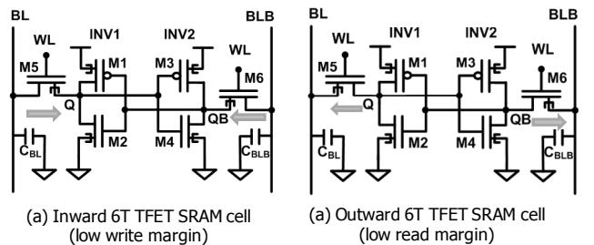
**Fig 12.** 6T TFET SRAM cell using TFET pass transistors pointing (a) inward and (b) outward. Inward 6T TFET SRAM has good read margin but poor write margin whereas the outward TFET SRAM exhibits excellent write margin but poor read margin.
