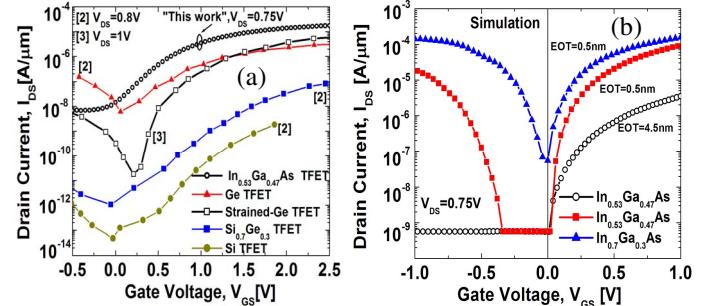
**Fig 10.** (a) Measured 100nm  $In_{0.53}Ga_{0.47}As$  TFET transfer characteristics showing highest  $I_{on}$  benchmarked against Si, SiGe, Ge and strained Ge TFETs. (b) Projected performance of  $In_{0.53}Ga_{0.47}As$  TFETs with EOT scaling and increasing indium content (70%) using calibrated TCAD model.
