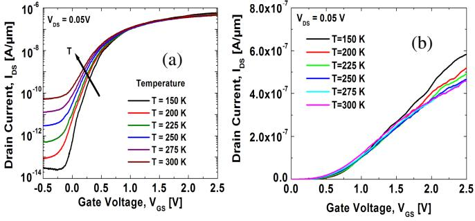
**Fig 7.**  $In_{0.53}Ga_{0.47}As$  TFET transfer characteristics illustrating the temperature dependence of the leakage floor and the on-current. The leakage floor increases exponentially with increasing temperature consistent with SRH generation recombination mechanism.
