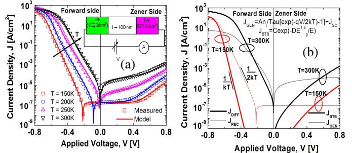
**Fig 3.** (a) Measured and modeled J-V characteristic and (b) various modeled components for  $\text{In}_{0.53}\text{Ga}_{0.47}\text{As}$  p+/i/n+ diode at various temperatures.
