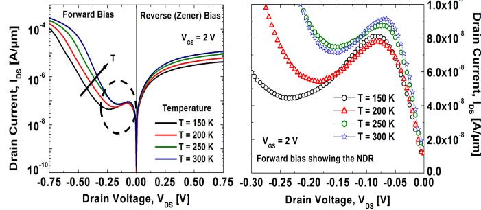
**Fig 9.** Gated negative differential resistance (NDR) characteristics as a function of temperature during forward bias between drain and source of  $In_{0.53}Ga_{0.47}As$  TFET. A PVCR of 2 is observed at 150K.
