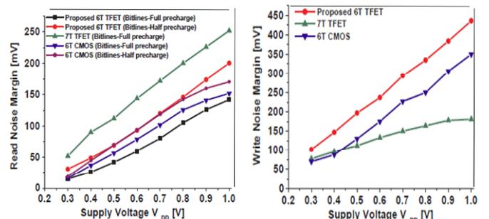
**Fig 14.** Excellent read and write noise margins achieved with the proposed 6T TFET SRAM cell with the SRAM cell exhibiting cell stability till 0.3V supply voltage.
