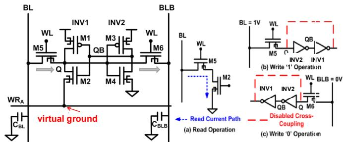
**Fig 13.** Novel 6T TFET SRAM is designed where M5 and M6 TFETs are used to write “1” and “0”, respectively, at node Q. During write, the cell is weakened by disabling the inverter pair cross-coupling via virtual ground. Read operation is similar to inward 6T TFET SRAM.
