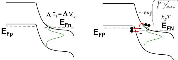
**Fig 6.** Energy band diagrams illustrating the impact of Dit on TFET sub-threshold slope; (a) Dit only effect is negligible and (b)  $D_{it}$  and TAT degrades sub-threshold slope since it involves tunneling into the interface traps and subsequent thermal emission from the traps giving rise to temperature dependence.
