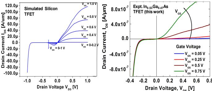
**Fig 11.** Asymmetric output characteristics in Si TFETs (simulated) and experimentally observed in  $In_{0.53}Ga_{0.47}As$  TFETs due to the inherent diode between source and drain, highlighting the difficulty in pass transistor implementation.
