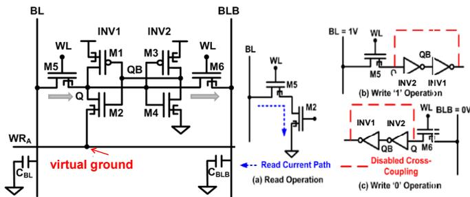
**Fig 13.** Novel 6T TFET SRAM is designed where M5 and M6 TFETs are used to write "1" and "0", respectively, at node Q. During write, the cell is weakened by disabling the inverter pair cross-coupling via virtual ground. Read operation is similar to inward 6T TFET SRAM.
