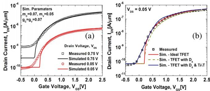
**Fig 4.** (a) Measured and simulated (ideal)  $\text{In}_{0.53}\text{Ga}_{0.47}\text{As}$  TFET transfer characteristics and (b) simulated transfer characteristics using the measured Dit as well as trap assisted tunneling (TAT) + Dit.
