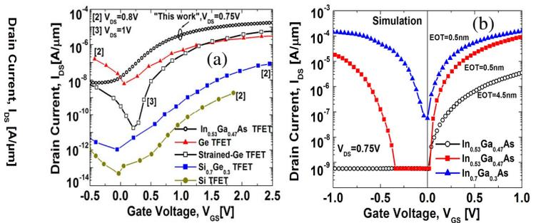
**Fig 10.** (a) Measured 100nm  $\text{In}_{0.53}\text{Ga}_{0.47}\text{As}$  TFET transfer characteristics showing highest  $I_{on}$  benchmarked against Si, SiGe, Ge and strained Ge TFETs. (b) Projected performance of  $\text{In}_{0.53}\text{Ga}_{0.47}\text{As}$  TFETs with EOT scaling and increasing indium content (70%) using calibrated TCAD model.
