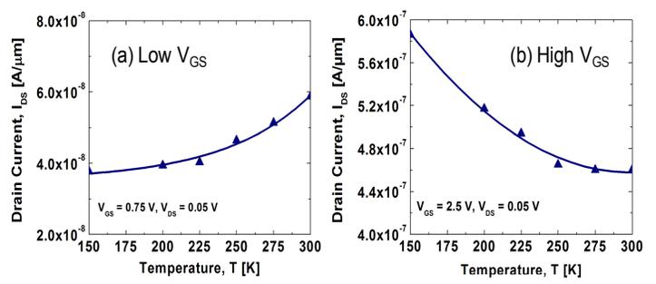
**Fig 8.**  $\text{In}_{0.53}\text{Ga}_{0.47}\text{As}$  TFET on current (a) increases at low  $V_{GS}$  due to reducing tunnel gap (limited by tunnel barrier resistance) and (b) decreases with temperature at high  $V_{GS}$  (limited by phonon scattering limited channel resistance).
