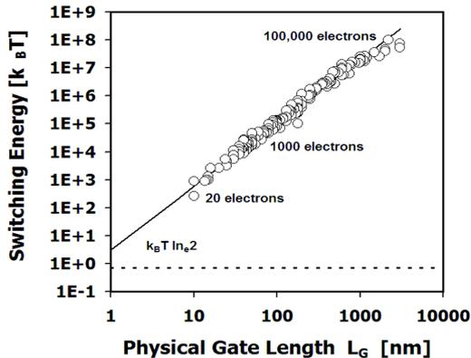
Fig. 1. Transistor switching energy plotted as a function of physical gate length. Also shown is the thermodynamic minimum energy for a hypothetical irreversible single particle binary logic gate [9, 10].
