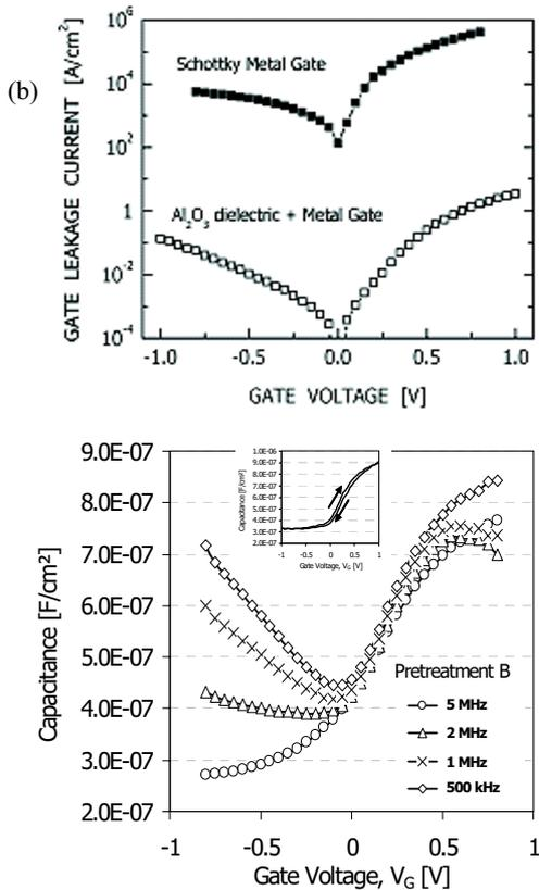
Fig. 5. Room temperature (a) gate to channel leakage characteristics for ALD Al<sub>2</sub>O<sub>3</sub> high-k dielectric and Al metal gate stack on AlInSb/InSb device layers showing four orders of magnitude reduction in leakage compared to Schottky metal gate (b) gate to channel capacitance characteristics showing frequency dispersion.
