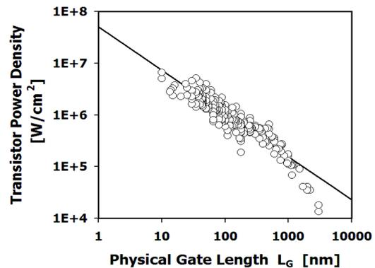
Fig. 2. Individual transistor switching power density plotted as a function of physical gate length. With physical dimensional scaling the device level power density continues to increase exponentially.
