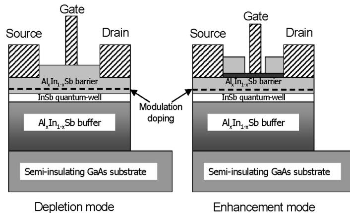
Fig. 3. Schematic of the depletion mode and enhancement mode indium antimonide (InSb) quantum well transistors.
