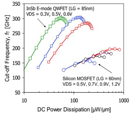
Fig. 7. Measured  $f_T$  vs DC power dissipation (normalized to the transistor width) for 85nm L<sub>G</sub> InSb QWFETs and 60nm L<sub>G</sub> silicon nMOS transistors.
