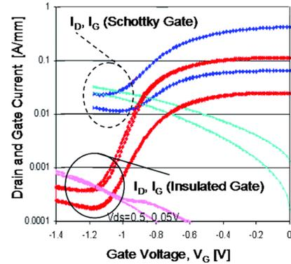
Fig. 6. Transfer characteristics of InSb QWFETs with Schottky metal gate and insulated metal gate with ALD Al<sub>2</sub>O<sub>3</sub> dielectric.
