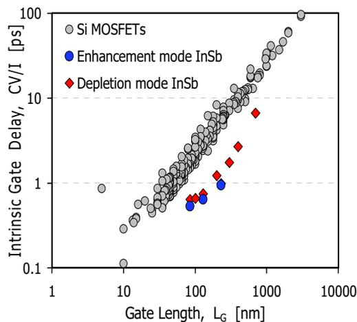
Fig. 8. Transistor gate delay (CV/I) versus gate length for InSb QWFETs at  $V_{DS} = 0.5$  V benchmarked against state-of-the-art silicon nMOS transistors.
