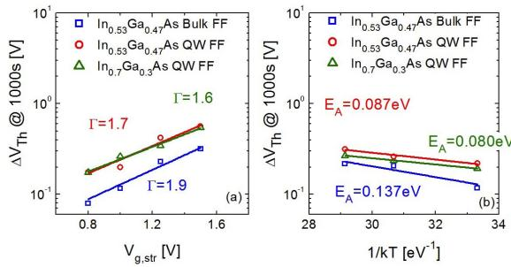
Fig. 5. (a) Plot of  $\Delta V_{Th}$  with respect to  $\Delta V_{g,str}$  to extract the voltage acceleration factor ( $\Gamma$ ) for the three architectures. (b) Plot of temperature activation of  $\Delta V_{Th}$  for the three architectures. The exponential fit gives us the activation energy,  $E_A$  values which are in accordance with the barrier height lowering due to quantization (fig. 1(c)).
