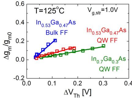
Fig. 4. Plot of  $\Delta g_m/g_{m0}$  with respect to  $\Delta V_{Th}$  for  $V_{g,str} = 1.0V$  at  $125\text{ }^{\circ}\text{C}$ .
