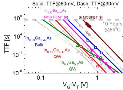
Fig. 6. Extrapolated times to  $60\text{mV}$   $\Delta V_{Th}$  (solid) at  $85\text{ }^{\circ}\text{C}$  operating temperature show that  $\text{In}_{0.7}\text{Ga}_{0.3}\text{As}$  QW FinFET needs to operate at  $0.1\text{V}$  of overdrive for 10 years of lifetime operation. The dashed lines are extrapolation of time to failure (TTF) at a more stringent  $\Delta V_{Th}$  of  $30\text{mV}$ .
