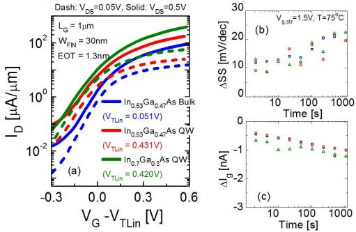
Fig. 2. (a) Transfer characteristics of the three FinFET architectures at gate length,  $L_G$ , of  $1\mu\text{m}$  considered in this letter. (b) and (c) shows degradation of SS and gate current,  $I_g$ , respectively for  $V_{g,\text{str}} = 1.5\text{V}$  and  $T = 75\text{ }^\circ\text{C}$  for the three architectures.
