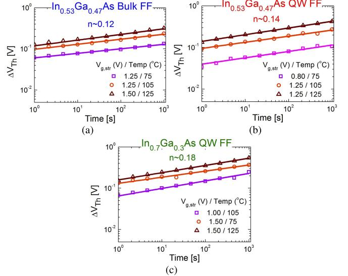
Fig. 3. Time evolution of  $\Delta V_{Th}$  under PBTI stress of different stress voltage,  $V_{g,\text{str}}$  and temperature,  $T$  for (a) In<sub>0.53</sub>Ga<sub>0.47</sub>As Bulk, (b) In<sub>0.53</sub>Ga<sub>0.47</sub>As QW, and (c) In<sub>0.7</sub>Ga<sub>0.3</sub>As QW FinFET devices, respectively. Using power law fitting based on eq.(1), the time exponent ( $n$ ) of each curve is extracted. The value of  $n$  for In<sub>0.53</sub>Ga<sub>0.47</sub>As Bulk architecture is the lowest.
