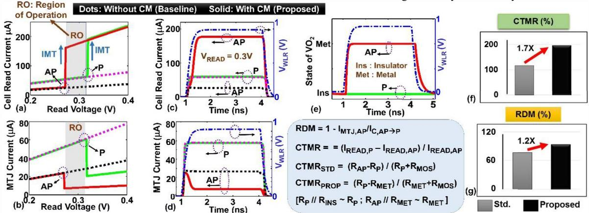
Fig. 3 (a) Read Voltage current of the cell and (b) MTJ current versus read voltage showing the region of operation (RO). Transient analysis showing (c) cell current, (d) MTJ current and (e) state of VO<sub>2</sub> during read. Substantial increase in the total cell current and reduction in the MTJ current for AP state leads to superior (f) cell TMR or CTMR and (g) read disturb margin (RDM) for the proposed MRAM cell compared to the baseline cell (existing multi-port MRAMs).
