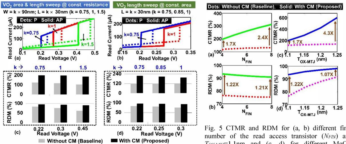
Fig. 4 Tuning of the region of operation and read voltage by changing (a) VO<sub>2</sub> area and length and (b) VO<sub>2</sub> length; (c, d) the corresponding comparison of CTMR and RDM for baseline and proposed cell.
