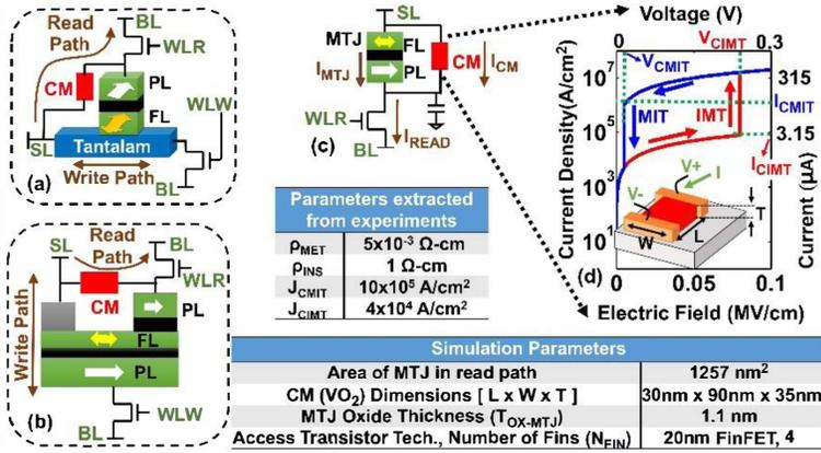
Fig. 1 (a, b) MRAM with separate read-write paths using the proposed technique of connecting a correlated material (CM) in parallel with the MTJ (c) Read equivalent circuit for the proposed MRAM cell (d) Characteristics of VO<sub>2</sub> (a CM) based on material parameters extracted from experiments.
