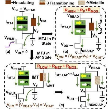
Fig. 2 Read operation of the proposed MRAM utilizing phase transition of the CM to enhance distinguishability and stability.
