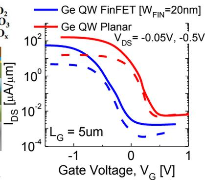
Fig2. IDVG comparison of Ge QW Planar with FinFET architecture shown in [1]
