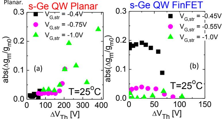
Fig6. absolute value of Normalized Transconductance degradation of (a) s-Ge QW Planar and (b) s-Ge QW FinFET. Planar devices' transconductance degrades with increasing stress while for FinFET it improves.
