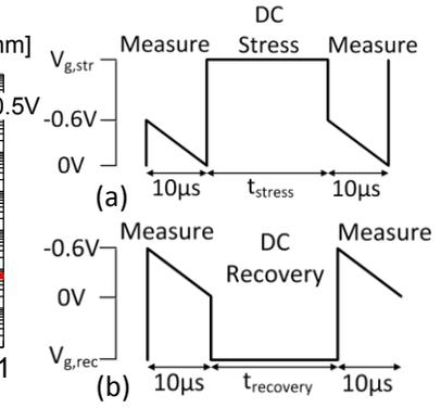
Fig3. DC Measurement schematic of Ultra Fast-MSM using Agilent B1530 Parameter Analyzer with measurement time of 10 $\mu$ s for (a) stress, and (b) recovery.
