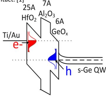
Fig4. Schematic Band Diagram of the gate stack under negative bias. Ge QW devices used in this study are dominated by electron trapping from gate electrode rather than hole from channel under NBTI.
