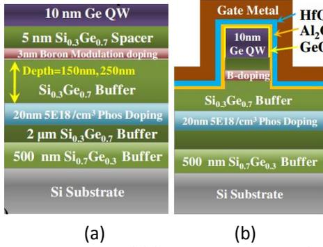
Fig1. Schematic of (a) s-Ge QW Planar wafer stack, and (b) FinFET stack with 25A HfO<sub>2</sub>/ 7A Al<sub>2</sub>O<sub>3</sub>/ 6A GeO<sub>x</sub> gate and Ti/Au gate metal contact. [1]
